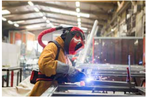
An example of personal fume extraction
